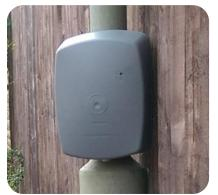
One tool to allow us to monitor usage of the routes are a number of beam-break electronic 'pedestrian counters' which are installed around the routes. For the latter two routes, Bicester West and Bicester North-East, these were installed a couple of months ahead of the line being in place, to allow us to have an idea of the background pedestrian traffic along the routes, and to therefore measure the increase once the route had been marked out.
